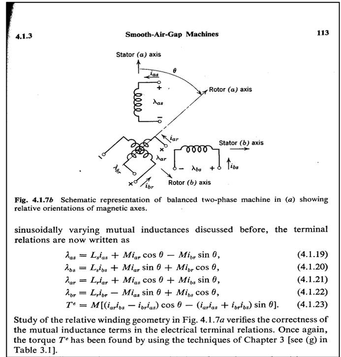
**Figure 1 - Herbert H. Woodson and James R. Melcher, “Electromechanical Dynamics, Part 1: Discrete Systems,” page 113, John Wiley & Sons, 1968.**
